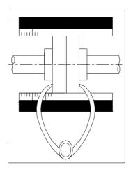
Figure 3 Aligning of the coupling for SM
