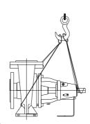
Figure 1 Lifting instruction pump set CP
